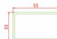
Door Reinforcing Steel
