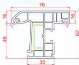
Outward Window Sash
