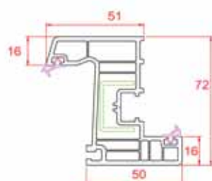
Narrow Window Sash
