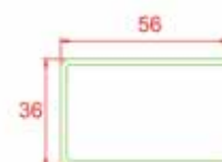
Door Sash Reinforcing Steel
