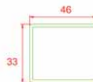
Narrow Door Sash Reinforcing Steel
